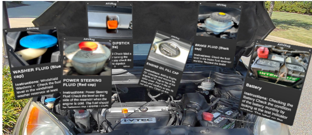
Fig. 4. Example of the AR interface for car component detection. The system identifies multiple engine components under the hood (e.g., washer fluid, power steering fluid, engine oil dipstick, brake fluid, engine oil fill cap, and battery) and overlays contextual retrieval cards containing both the component label and step-by-step maintenance instructions, as well as sample images retrieved from the database. The controller-defined planar window allows the user to select an object for identification in real-time.
