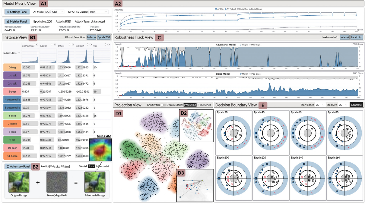
Fig. 2. The ATVis interface comprises five key components. (A1) Quantitative metrics and (A2) the accuracy line chart provide an overview of model performance. (B1) The instance table view and (B2) adversarial attack demonstration offer detailed instance-level insights. (C) Area charts track robustness during training. (D1, D2, D3) t-SNE projections in the embedding space reveal distribution patterns, and (E) the decision boundary view allows dynamic inspection of boundary changes.
